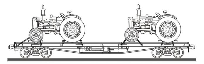
12. You will note that they have been positioned so that the front wheels of one tractor and the rear wheels of the other tractor have been positioned over the center of the bogie bolsters.
